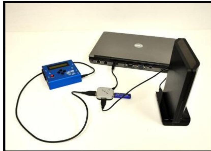
**Use USB Hub is the computer has less than 4 USB ports**
